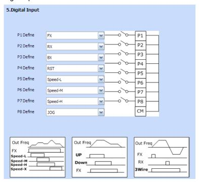
Set the parameters corresponding to Digital Input.
