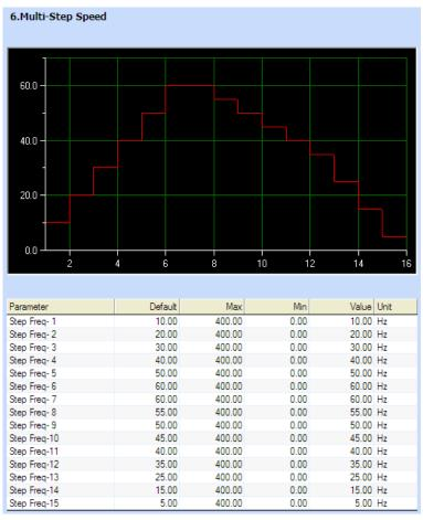
Set the parameters corresponding to Set Multi-Step Speed.
