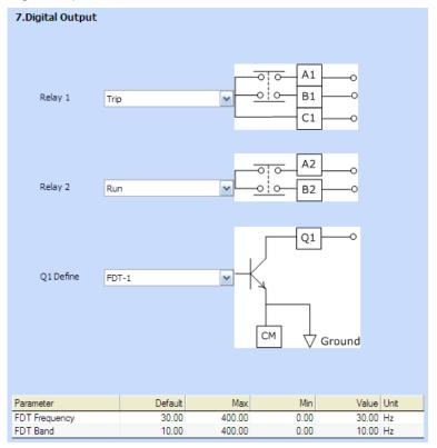
Set the parameters corresponding to Digital Output.
