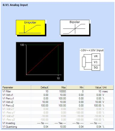
Set the parameters corresponding to V1 Analog Input.
