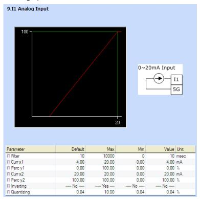
Set the parameters corresponding to I1 Analog Input.
