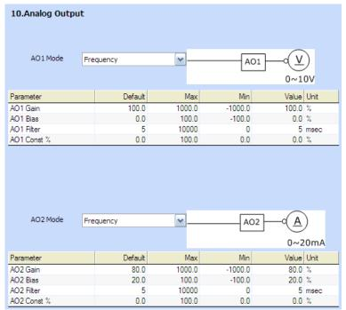
Set the parameters corresponding to Analog Output.
